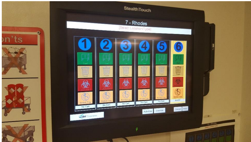
Image 2- Control panel used to signal a robotic vehicle to transport a specific type of waste to the waste disposal facility
