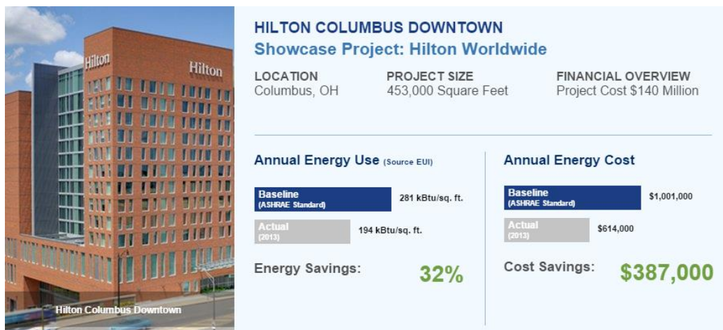
Figure 6. This image shows the energy and cost savings this building has reached after completion of the project. Publicizing this information will make this information can energy efficiency more attractive to consumers.
